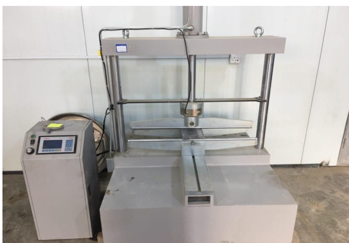
Figure 6 Tester device for flexural testing.
