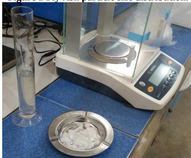
Figure 3 Soluble sodium silicate and sodium hydroxide pellets.
