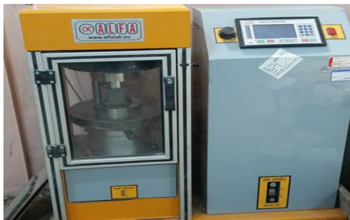
Figure 5 The compressive machine.
