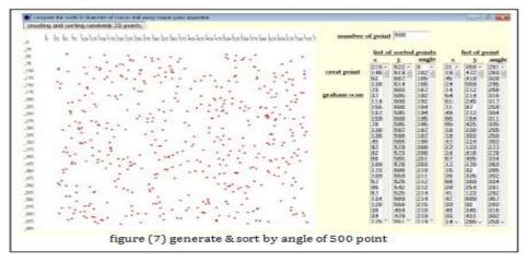
**Second:**Sort the points by angles in counter clockwise order using equation number(3,4) represents the mergsortalgorithmsteps, in the same time the two dimension points are also rearrange according to value of angle belongs to eachpoint. Finally we draw line between anchor point and all othersorted points to show thearrangement of points as shown in figure (8)
