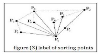
**Step7:** Remove right turn point If the inner angle formed by Pa, Pb,Pc is greater than or equal to 180° then we eliminate the point labeled with Pb. Setpoint Pb to be
