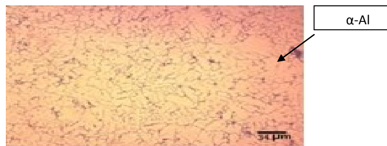
Figure 2: The microstructure of base alloy.
