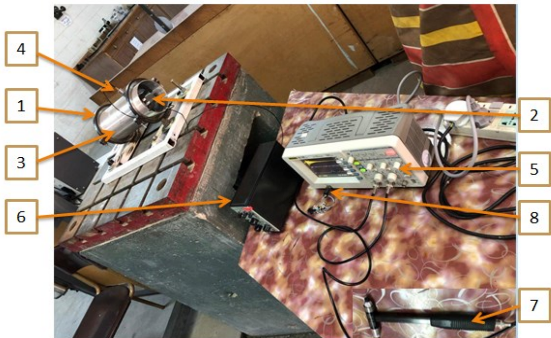
Figure 5: SS-SS Cylindrical shell vibration test rig.
