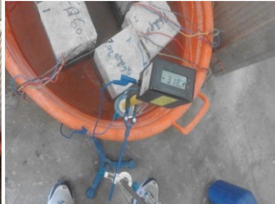
Fig. 5 Half-cell potential test
