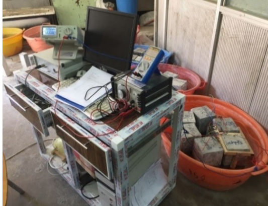
Fig. 3 AC resistance test
