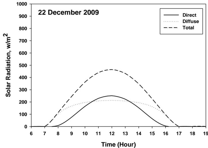
Figure 4: Direct, diffuse, and total solar radiation components during winter solstice for Tikrit city.
