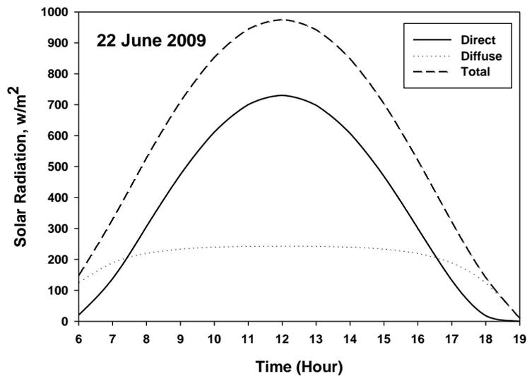
Figure 2: Direct, diffuse, and total solar radiation components during summer solstice for Tikrit city.
