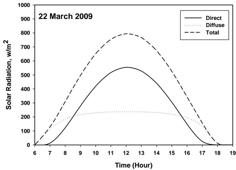
Figure 1: Direct, diffuse, and total solar radiation components during spring equinox for Tikrit city.
