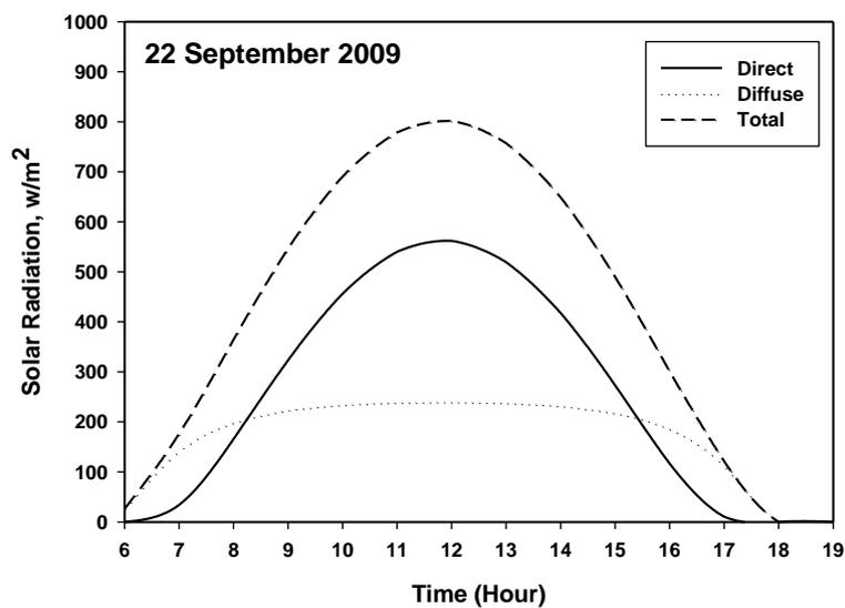
Figure 3: Direct, diffuse, and total solar radiation components during autumn equinox for Tikrit city.
