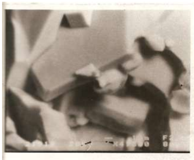
Figure(6)Morphology of fracture surface of compound (YBa 2 Cu 3 O 7+δ )
