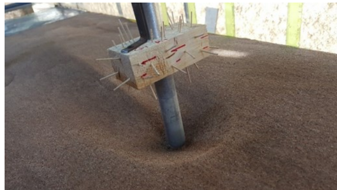
Figure 6: Scour hole of debris accumulation of group 1, L_d/D=2 and T_d/D=0.5 .
