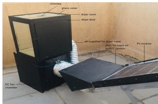
Figure 1: Component of the PVT system to dryer solar system.
