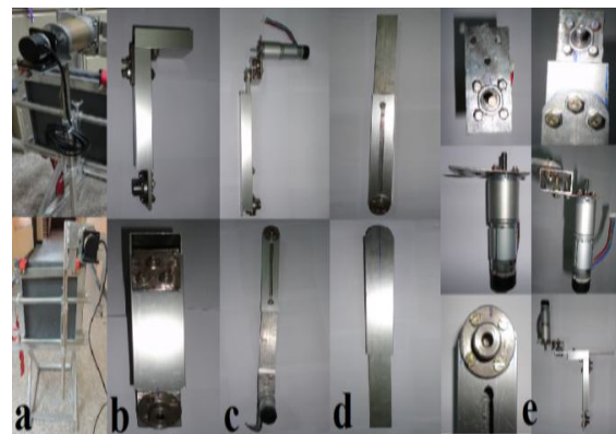
Figure 5. (a) The robot base. (b) The first and second links. (c) The third link. (d) The fourth link. (e) Motors bases, Flanges and other finishing's.
