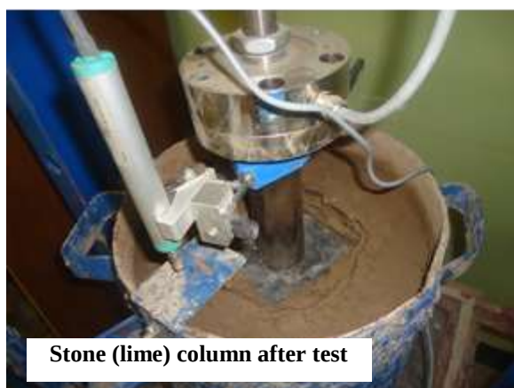
Figure (3) : Stone (Lime) columns before and after tests
