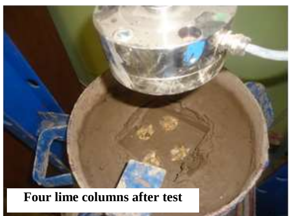
Figure (3) : Stone (Lime) columns before and after tests
