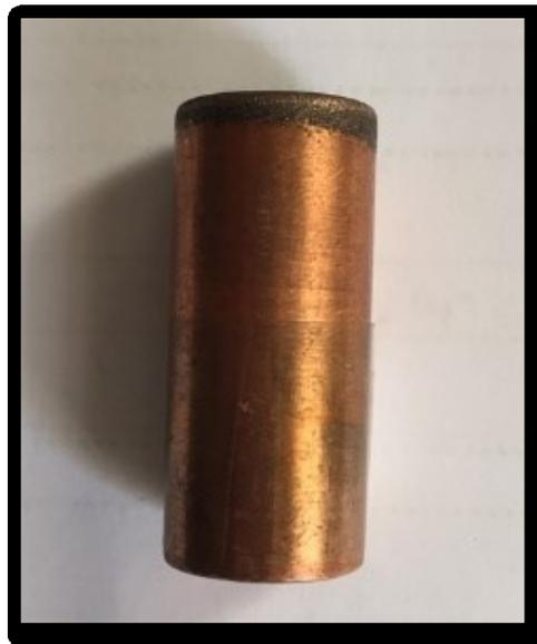
Figure 3: The tool (Electrode).
