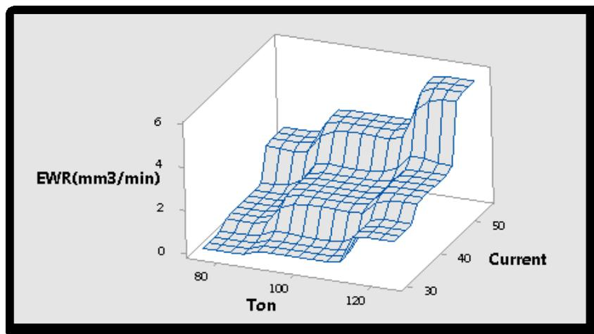
**Figure 7: Plot of Surface of Electrode Wear Rate (mm<sup>3</sup>/min) vs Current; Ton**
