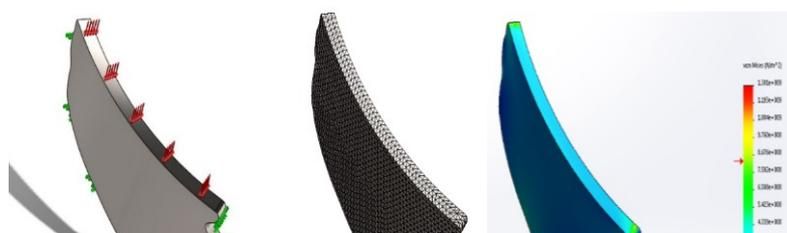
**Figure 5: (a) mesh model of the implant. (b) Directional constraints (c) Color-coded analysis**
