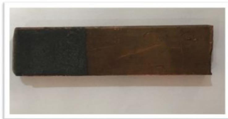
**Figure 3: The copper electrode.**
