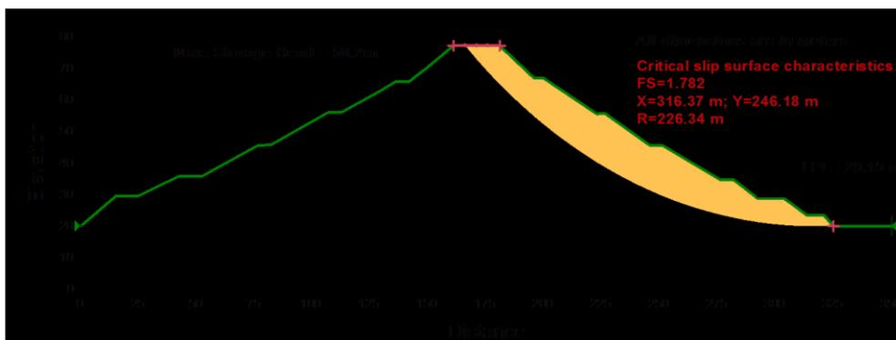
**Figure 14: Critical slip surface position for the downstream slope for the in situ layers**
