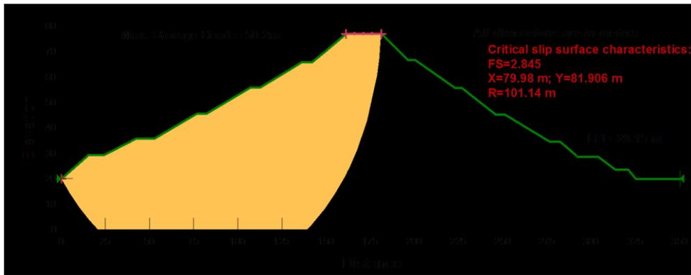
Figure 15: Critical slip surface position for the upstream slope for the gypseous layers
