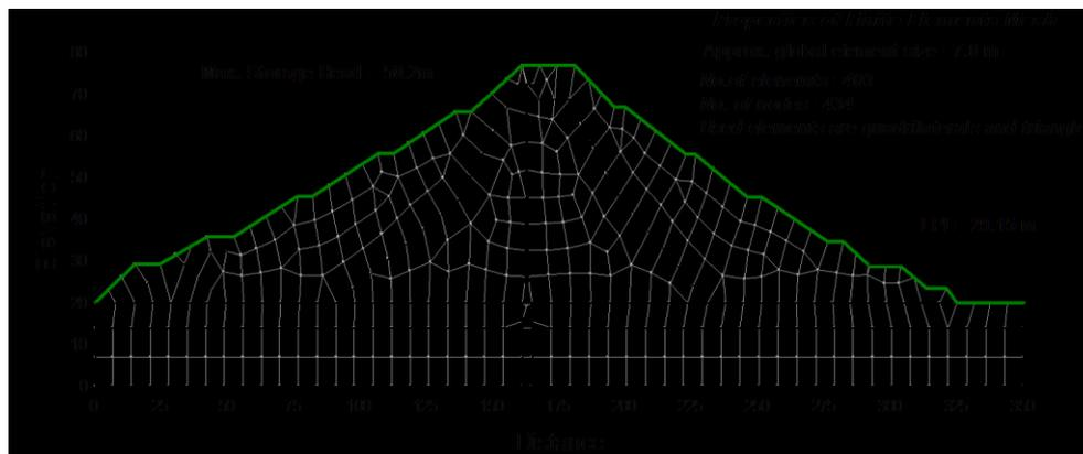
**b) Discretization of the Finite elements mesh of the dam cross-section**
