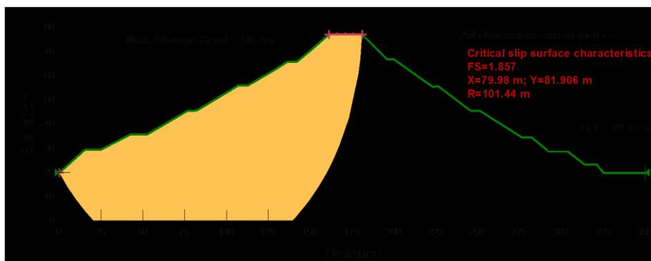
**Figure 13: Critical slip surface position for the upstream slope for the in situ layers**
