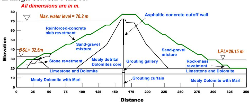
The zones of the dam and its foundation with their materials and finite elements mesh characteristics are shown in Figure 2.
