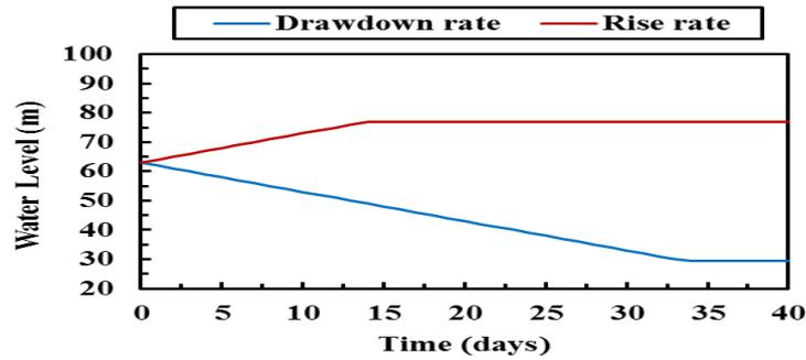
Figure 8: Hypothetical drawdown and rise rates of water level in the dam reservoir
