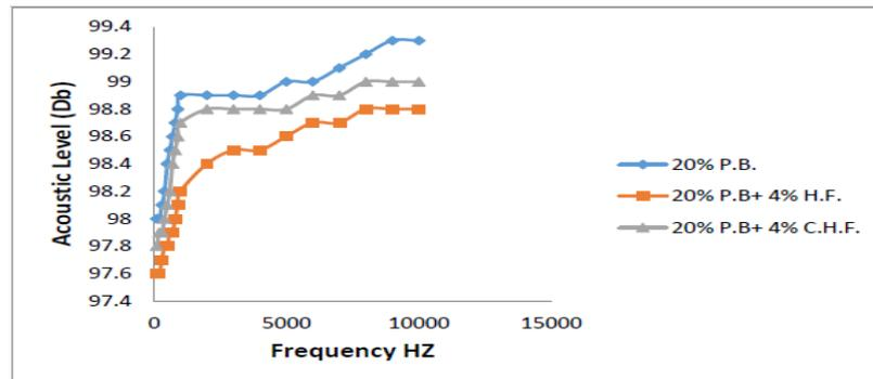
Figure 8: Acoustic level with a frequency with Weight Fraction of 20% P.B reinforcing with 4% (hemp fibers H.F., cornhusk fibers C.H.F.).
