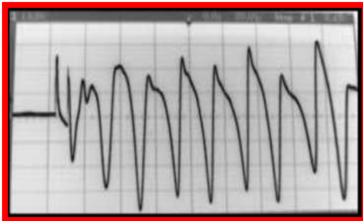
Fig(8)The voltage build up at a prime for a prime mover speed of 1180 rpm mover speed of 1115 rpm
