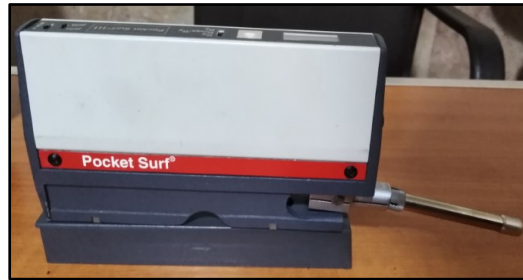
Figure 3: The surface roughness tester (Pocket Surf)
