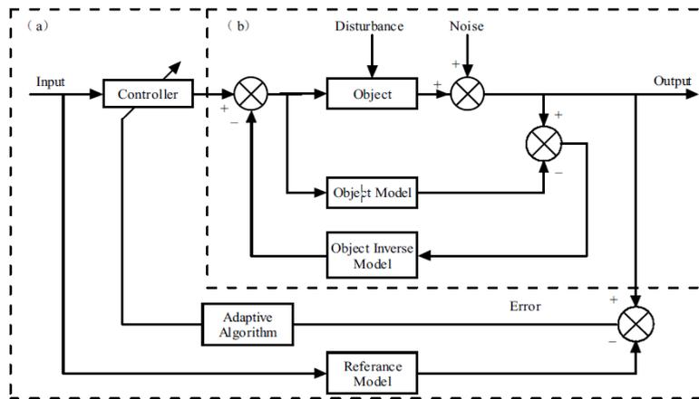
Figure 2 the structure system of adaptive inverse control [6]
