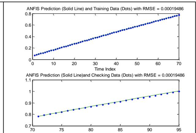
Figure 11 simulation result using ANFIS for training and checking data of E-W position
