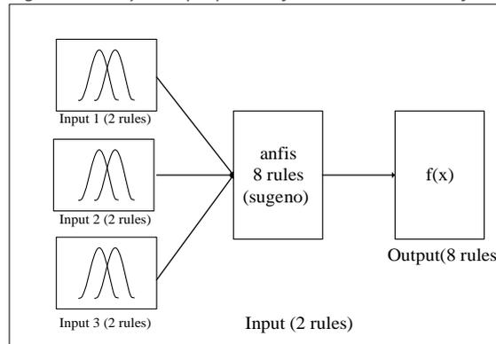
Figure 5 The system diagram of ANFIS
