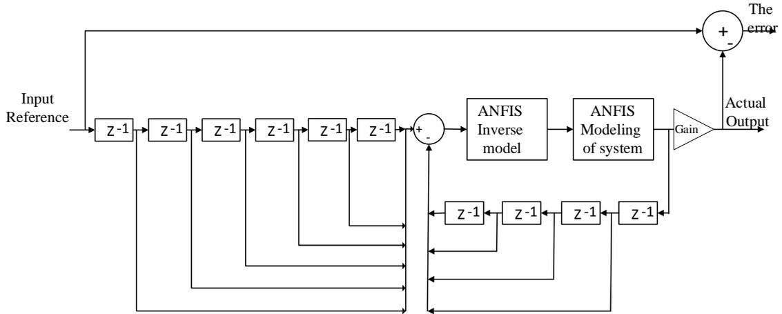
Figure 4 The system proposed of radar tracker identification
