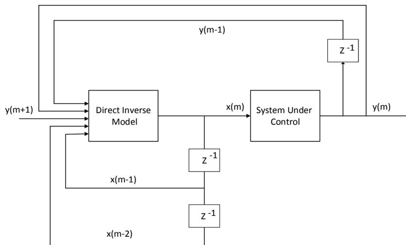
Figure 3 structure of the direct inverse control
