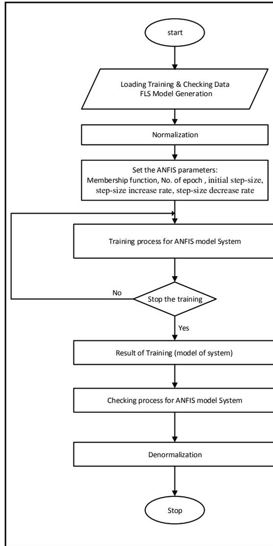
Figure 12 The flowchat of ANFIS trainings and checking for identifications processes.
