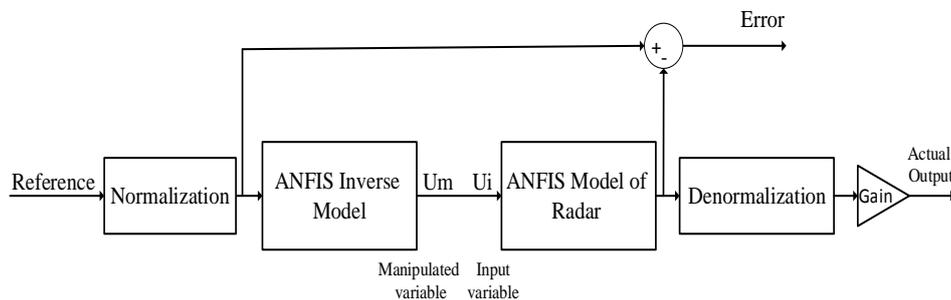
Figure 13 proposed system of aircraft position radar system on inverse modeling design
