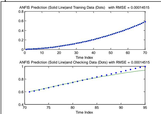
Figure 8 checking and training results with ANFIS prediction of inverse modeling of N-S position
