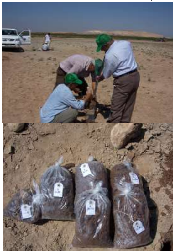
Figure 3: Field collection of samples by using hand auger
