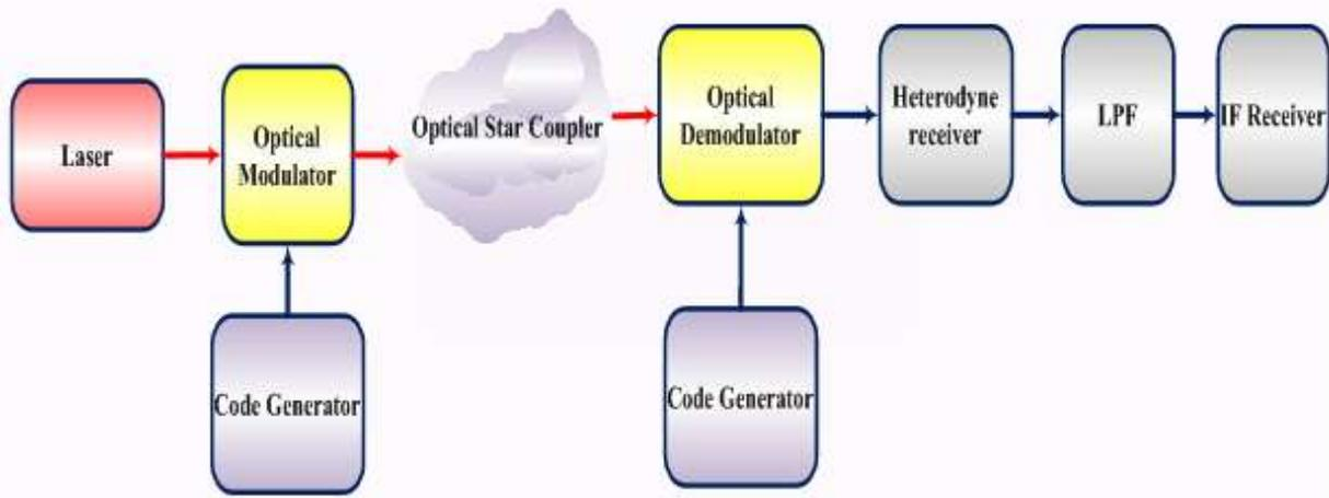
Fig. 4: OCDMA encoder/decoder structure.
