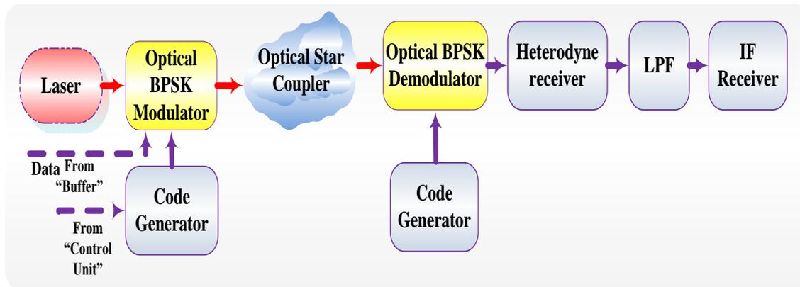
Fig.5 OCDMA encoder/decoder scheme.
