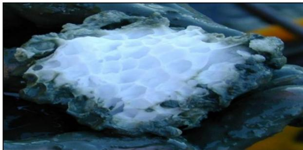
Figure 1: Crystal forming of Clathrate-hydrate [17]
