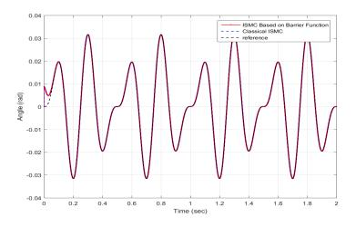
Figure 10: Angle  $x_1$ vs. time using saturation function for Classical ISMC,  $T_L$  = variable.
