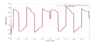
Figure 8: The control input u vs. time using saturation function for Classical ISMC,  $T_L$  = constant.
