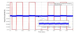
Figure 3: The integral sliding manifold s(t) vs. time,  $T_L$  = constant.
