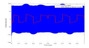
Figure 4: The control input u vs. time using saturation function for Classical ISMC,  $T_L$  = constant.
