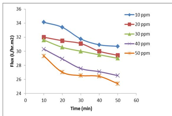
Figure 6: Effect of feed concentration on the permeate flux of PVC membrane (TMP=1bar, feed flow =100mL/min)
