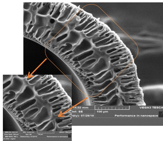
Figure 3: SEM image of the PVC membrane
