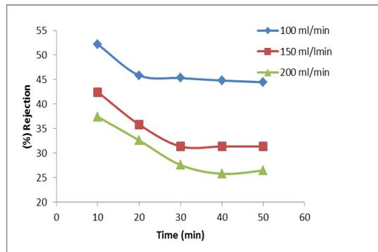
Figure 5: Effect of feed flow rate on the rejection of MG dye (TMP=1bar, feed concentration=100mg/L)
