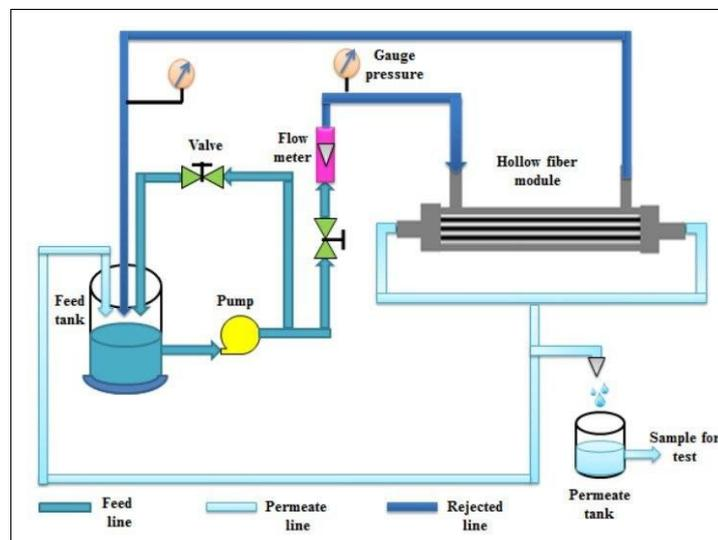
Figure 2: Schematic diagrams of the UF experiments set-up
