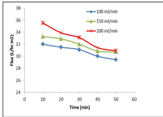
Figure 4: Effect of feed flow rate on the permeate flux of PVC membrane (TMP=1bar, feed concentration=100mg/L)
