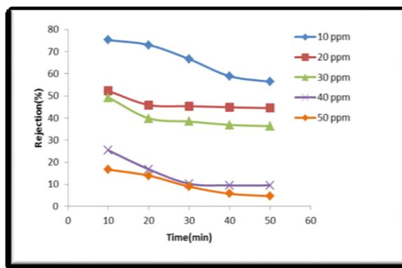
Figure 7: Effect of feed concentration on the rejection of the hollow fiber membrane (TMP=1bar, feed flow =100mL/min)
