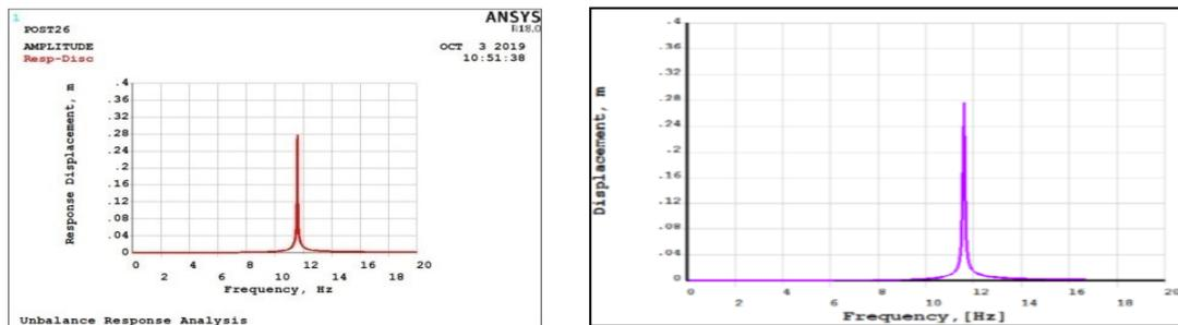
**Figure 1: Unbalance response a: ANSYS software, b: [9]**
