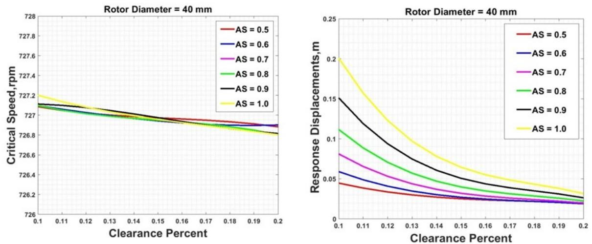
Figure 5: Effect of bearing clearance on the response and critical speed
