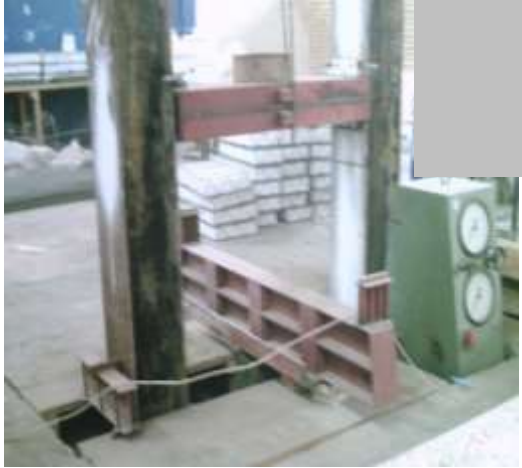
Fig. 4: Compressive testing machine
