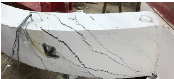
Fig. 9 Specimen C3 failure.
