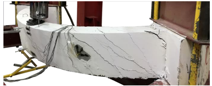
Fig. 10 Specimen C4 failure.
