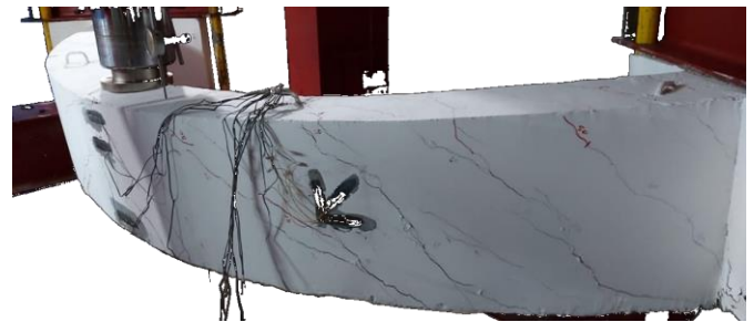
Fig. 11 Specimen C5 failure.
