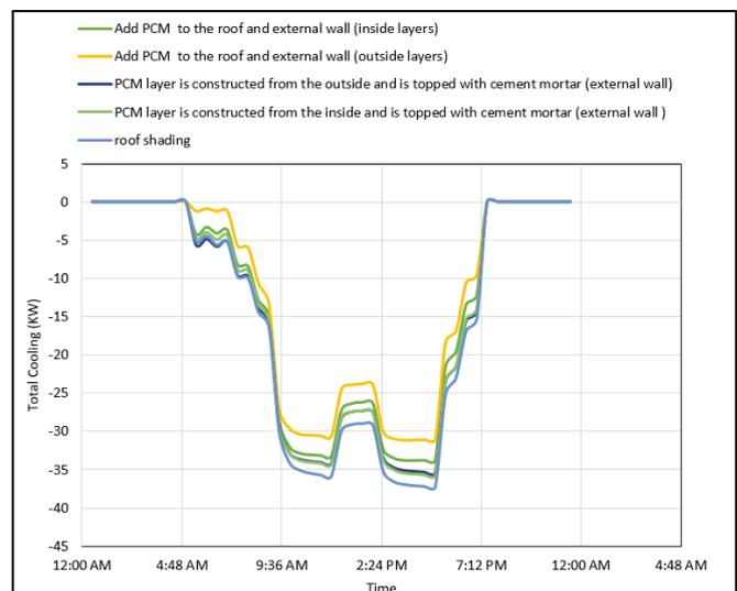
**Fig. 11** Total cooling load with time in July.
