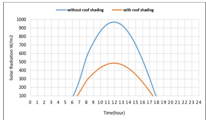
**Fig. 10** Solar radiation without roof shading and with roof shading.
