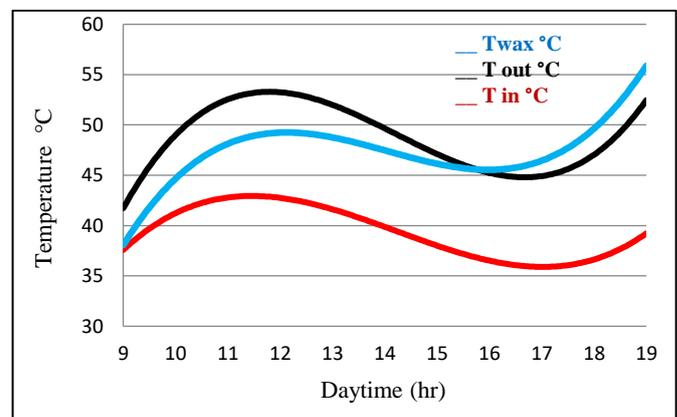
Fig. 6 Collector performance vs daytime with tank flow rate 4 L/min collector flow rate 4 L/min (1<sup>st</sup> Sep 2021).
