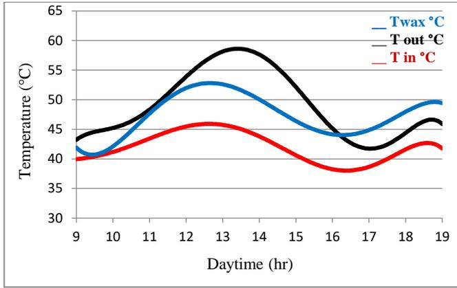
**Fig. 7** Collector performance vs daytime with tank flow rate 4 L/min collector flow rate 4 L/min (1<sup>st</sup> April 2022).
