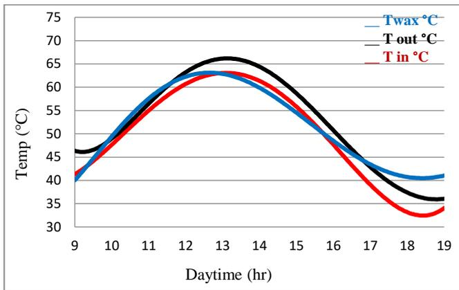
**Fig. 8** Collector performance vs daytime with tank flow rate 4 L/min collector flow rate 4 L/min (1<sup>st</sup> May 2022).
