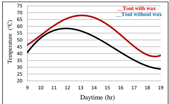
**Fig. 11** Experimental outlet collector temperature with and without wax (May 2022),  $V_{in} = 4$  L/min,  $T_{in} = 25$  °C.
