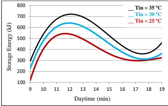
**Fig. 18** Thermal storage for the storage tank with different inlet water temperature,  $V_{in} = 2 \text{ L/min}$ , (1<sup>st</sup> May 2022).
