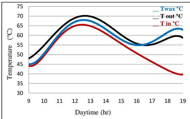
**Fig. 9** Collector performance vs daytime with tank flow rate 4 L/min, collector flow rate 4 L/min (1<sup>st</sup> June 2022).
