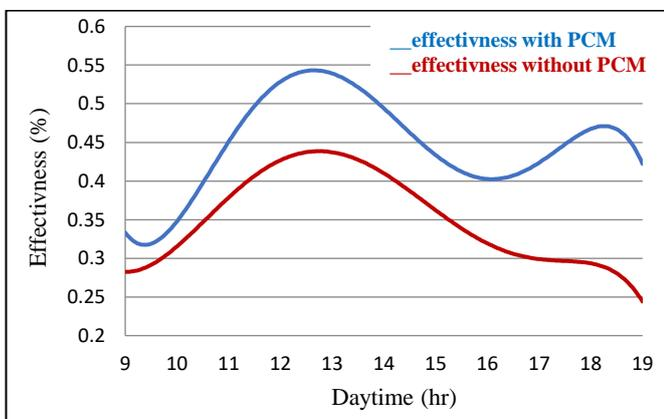
**Fig. 20** Comparison results for heat exchanger effectiveness with and without PCM VS daytime,  $V_{in} = 2 \text{ L/min}$ ,  $T_{in} = 25 \text{ °C}$ . (1<sup>st</sup> May 2022).
