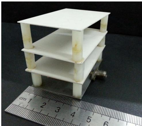
Figure 4. Fabricated multilayer antenna.
