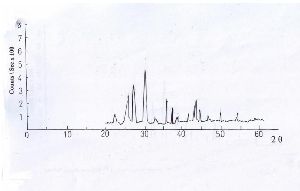
Fig(A-1):X-ray diffraction of  $(\text{Bi}_2\text{Ba}_2\text{Ca}_2\text{Cu}_3\text{O}_{7-\delta})$  at  $(790)^\circ\text{C}$
