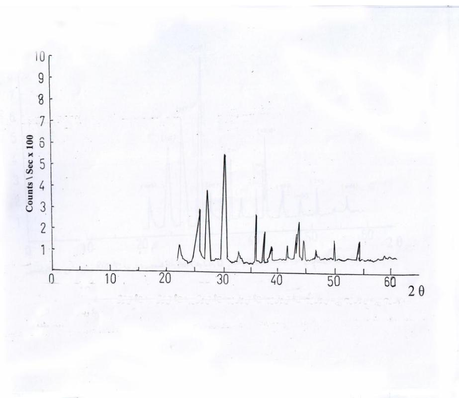
Fig(A-2):X-ray diffraction of  $(\text{Bi}_2\text{Ba}_2\text{Ca}_2\text{Cu}_3\text{O}_{7-\delta})$  at  $(830)^\circ\text{C}$
