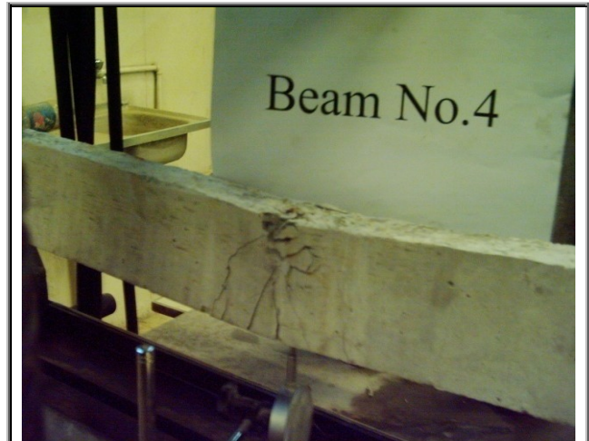
Plate (4) Typical non-composite beam at failure (yield of bottom steel reinforcing bars with excessive tension cracks converging the top surface)
