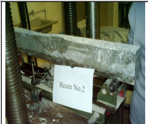
Plate (3) Typical composite beam at failure (crushing of concrete in compression zone at the middle one-fifth of the simple span)
