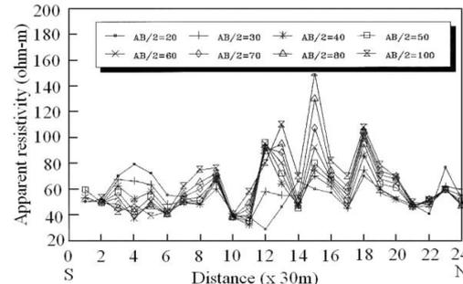
Fig.3 Apparent resistivity profiles at different electrode spacing
