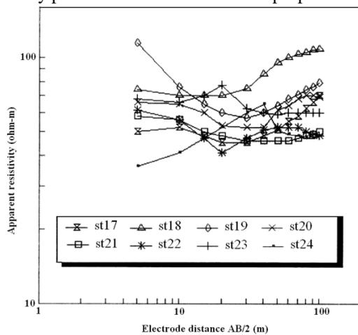
Fig.4 Some of the field resistivity (VES) curves
