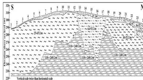
Fig.5 Geo-electrical cross-section along the traverse
