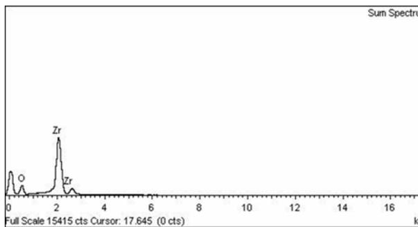
**Fig.6,** EDX image of ZrO<sub>2</sub>/Nps.
