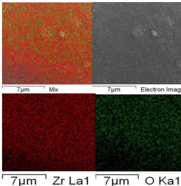
**Fig.7,** Spectral analysis (EDX) of ZrO<sub>2</sub>/Nps.
