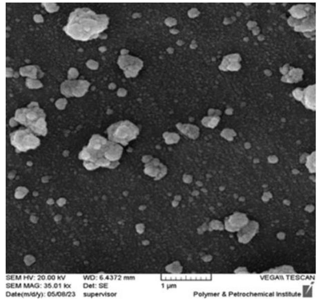
**Fig.4A,** The SEM image of ZrO<sub>2</sub>/Nps.
