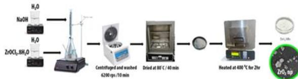
**Fig.1,** The preparation Steps to ZrO<sub>2</sub> nanoparticle.
