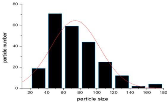
**Fig.5,** The particle size distribution of (ZrO<sub>2</sub>)/Nps.
