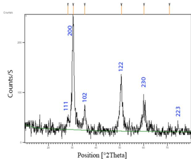
**Fig.2,** The XRD spectrum of ( $ZrO_2/Nps$ ).
