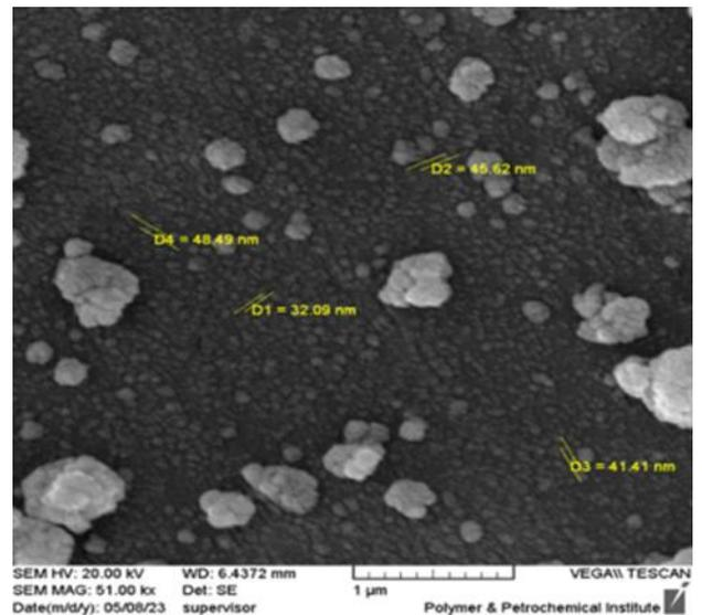
**Fig.4B,** The SEM image of ZrO<sub>2</sub>/Nps.
