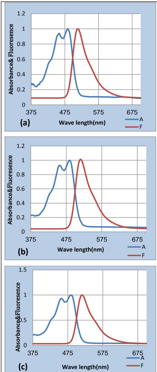
Figure 11: Spectra of absorption (A) and fluorescence (F) of the mixing fluorescein sodium dye and nanoparticles of Zinc acetate at different concentrations [(a)  $2 \times 10^{-5}$  (b)  $7 \times 10^{-5}$  (c)  $1 \times 10^{-4}$ ] mol/L.
