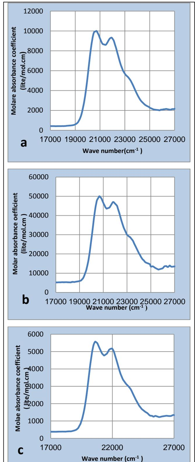
Fig 12: Spectra of molar coefficient ( $L/mol.cm$ ) versus Wave number ( $cm^{-1}$ ) fluorescein sodium dye at different concentration [ (a)  $1 \times 10^{-4}$ , (b)  $2 \times 10^{-5}$ , (c)  $7 \times 10^{-7}$  ] mol/L.
