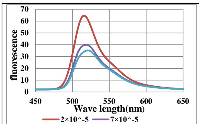
**Figure 8:** fluorescence spectrum of fluorescein sodium dye at different concentrations.
