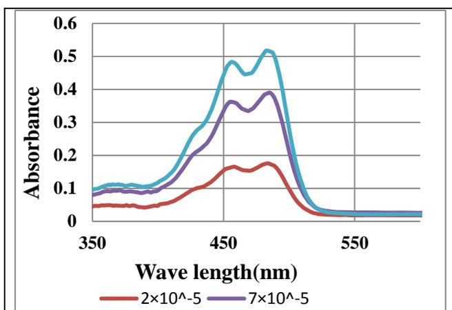
**Figure 9 :** Absorption spectrum of mixture dye and nanoparticles of zinc acetate at different concentrations.
