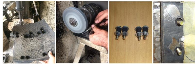
Figure 2: Process of the covered bolts by rubber
