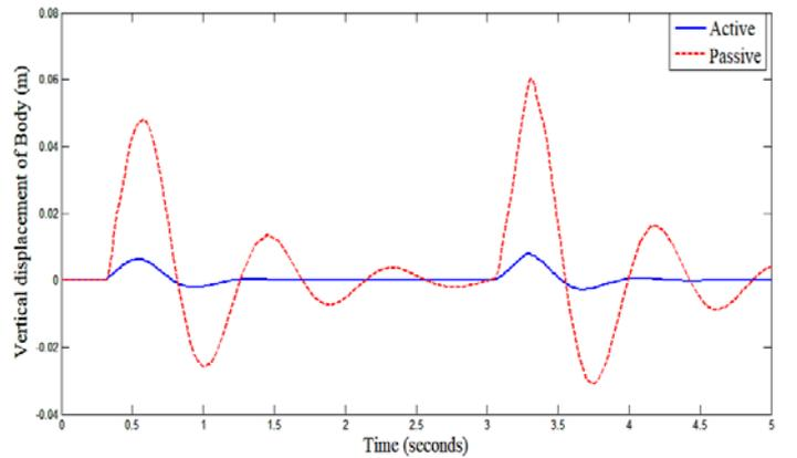
Fig. 12 Body Displacement (Case 2)
