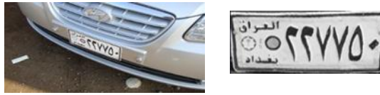
Figure 15: The application of affine transform to correct plate shearing issues: (a) original image, and (b) obtained image after applying an affine transform.
