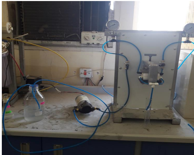
Figure 2 : Photograph image for the ultrafiltration system
