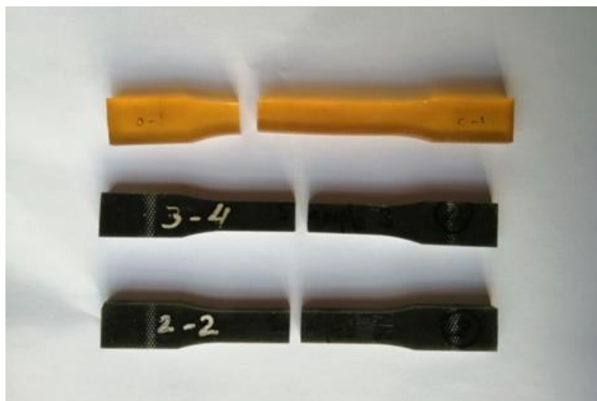
Fig. 10 Mode of fracture.
