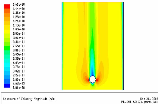
**Fig.(7) Velocity distribution around the cylinder  $Re = 2274$**
