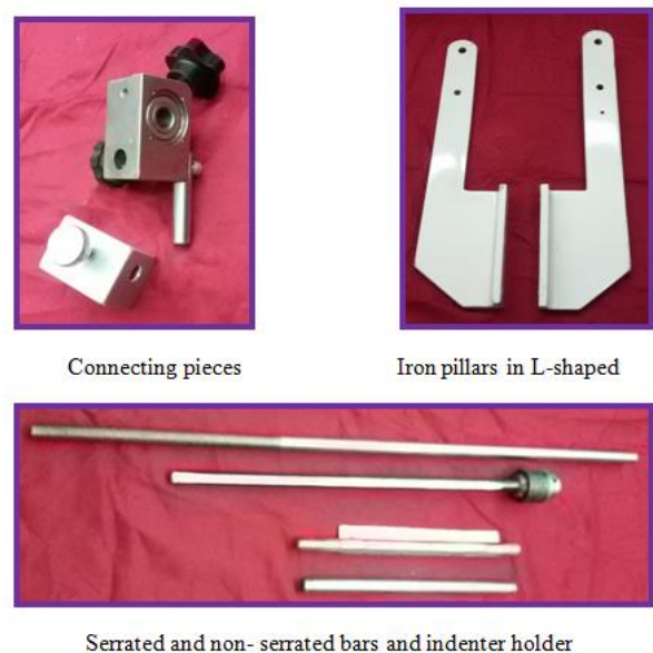
Fig. 3 Scratching mechanism parts.
