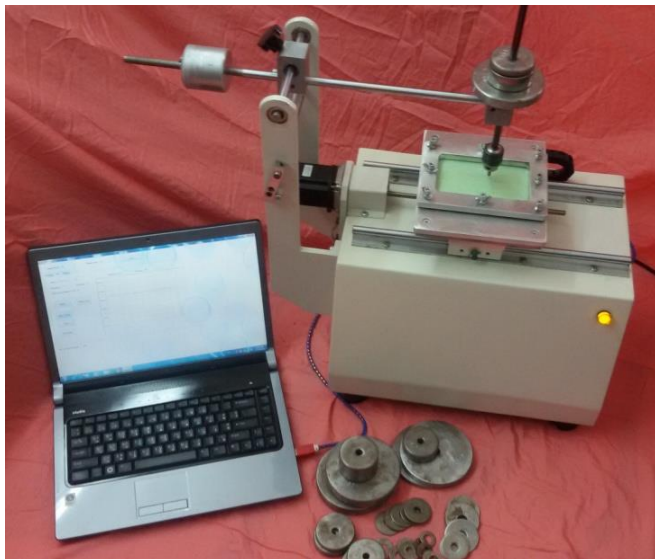
Fig. 1 Scratch resistance device.
