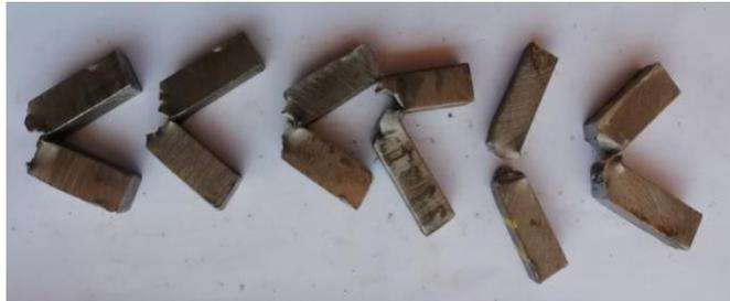
Fig. 4 Impact specimen after test.
