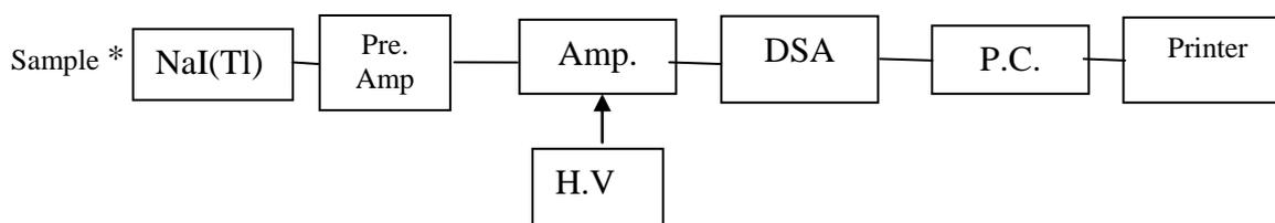
**Fig.3: Shows the schematic diagram of the setup.**
