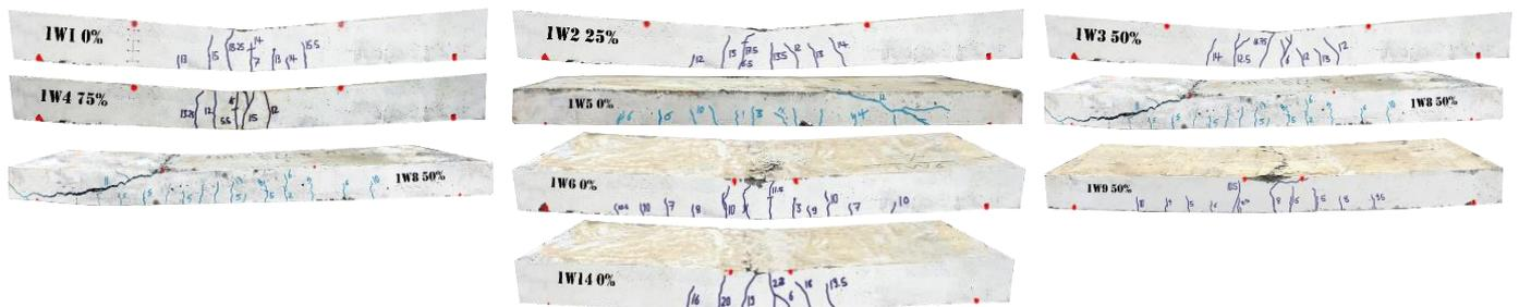
**Fig. 6** Cracks pattern of slabs failed in flexure.
