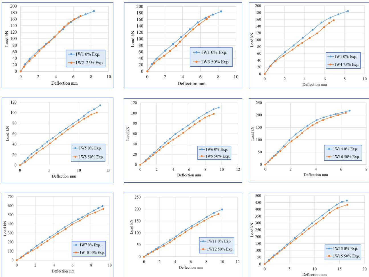
Fig. 5 Experimental load versus mid-span deflection curve Slabs.
