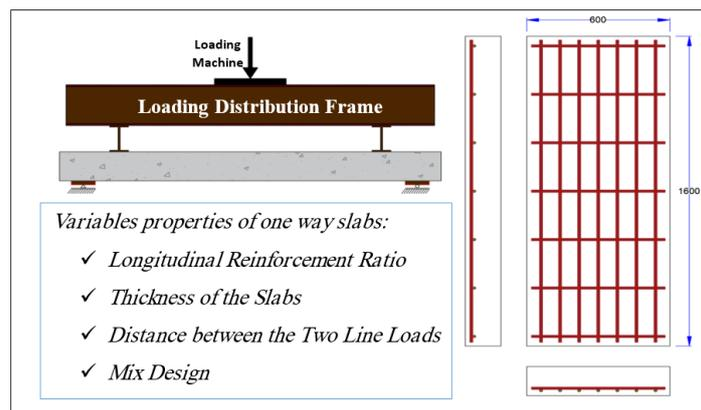
Fig. 2 Slabs Details and considered loading system.
