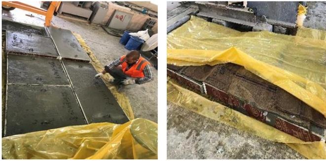
Fig. 3 Concreting and curing the slabs.
