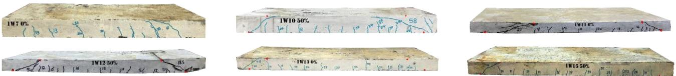
Fig. 8 Cracks pattern of slabs failed in shear.
