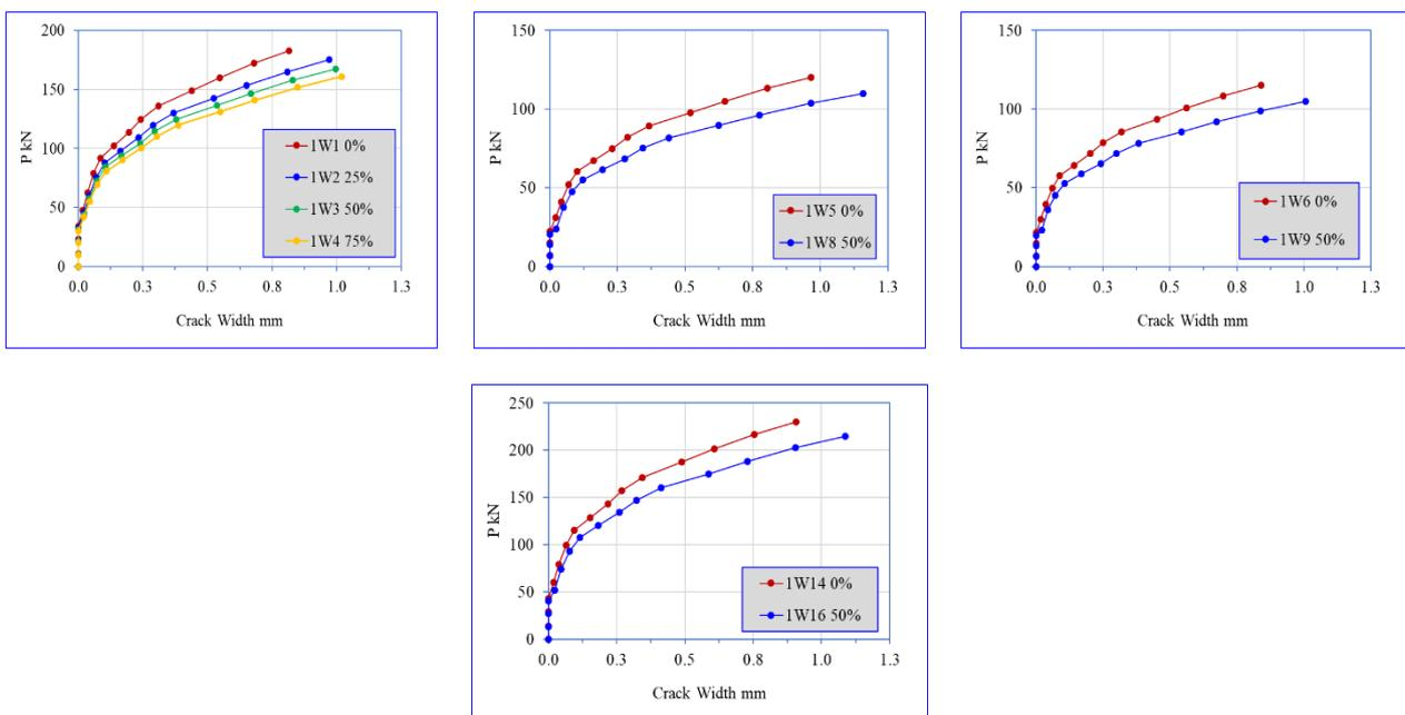
**Fig. 7** Load-flexural cracks relations for slabs failed in flexure.
