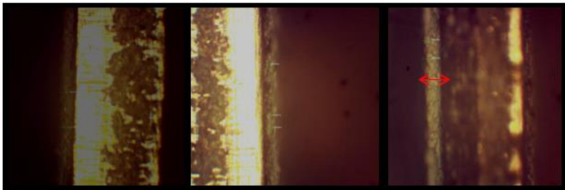
Figure 3: Computerized optical microscope measurement shows the coating thickness at the interface of PMMA- based composite coating by electrostatic technique: A (6% \text{Al}_2\text{O}_3 and 4% \text{TiO}_2 with 90%PMMA) B (9% \text{Al}_2\text{O}_3 and 6% \text{TiO}_2 with 85%PMMA) and C (12% \text{Al}_2\text{O}_3 and 8% \text{TiO}_2 with 80%PMMA), at magnification 40X
