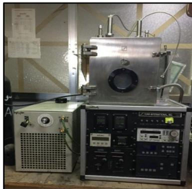
Figure 1: RF Magnetron sputtering system.
