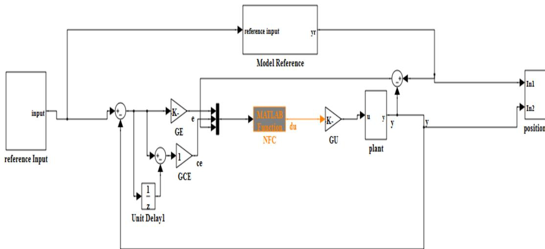
**Figure (2): MATLAB/Simulink block diagram for Neuro-Fuzzy Model Reference Adaptive Control**
