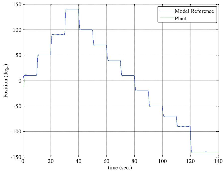
Figure (8): step response for all operation point.
