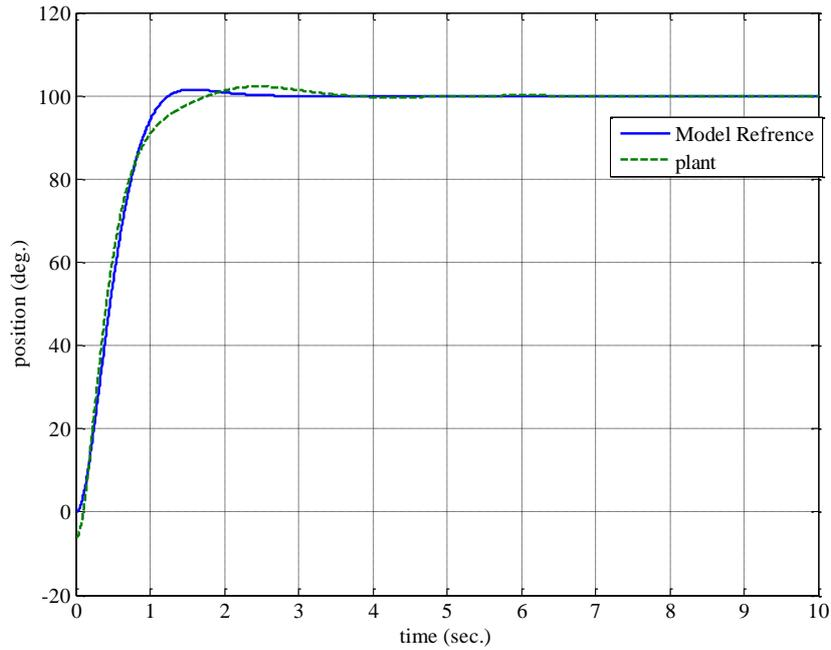
**Figure (5): step response for 100 Deg.**
