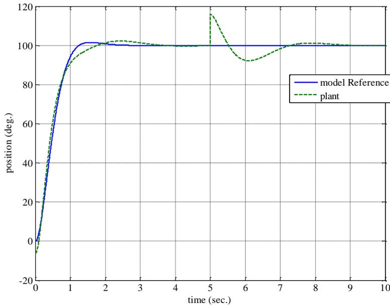
**Figure (6): step response for 100 Deg. with parameter variation at 5 sec.**
