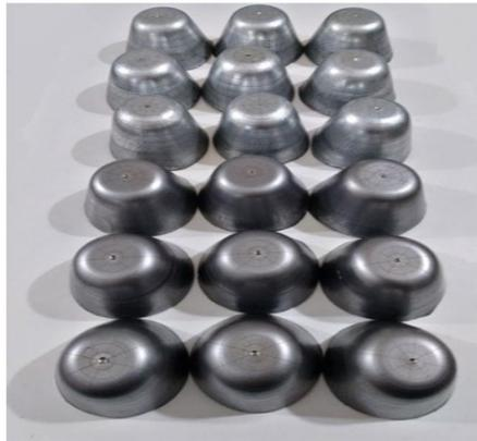
**Figure 6: Photographs show the cups produced from different die wall angles, punch velocities, material types, and sheet thicknesses.**
