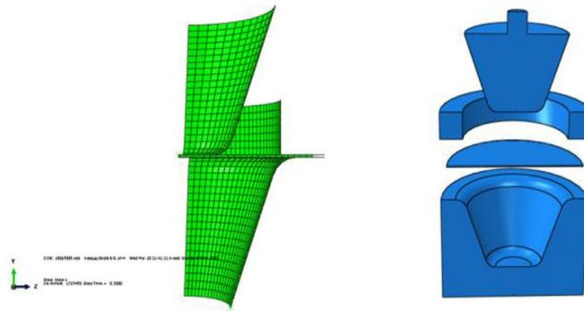
Figure 7: Assembled model meshed using ABAQUS 6.14.
