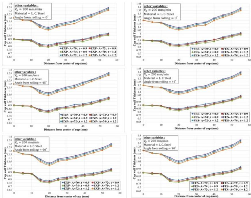
Figure 15: Effect of die wall angle variation in thickness behavior of low carbon steel at 200 mm/min punch velocity and 0.9 & 1.2 mm thickness along 0°, 45° and, 90° directions experimentally and numerically.
