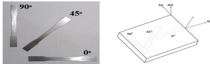
Figure 2: Tensile test specimens according to the rolling direction.
