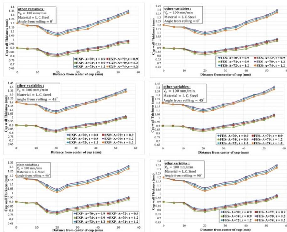
Figure 11: Effect of die wall angle variation in thickness behavior of low carbon steel at 100 mm/min punch velocity and 0.9 & 1.2 mm thickness along 0°, 45° and, 90° directions experimentally and numerically.
