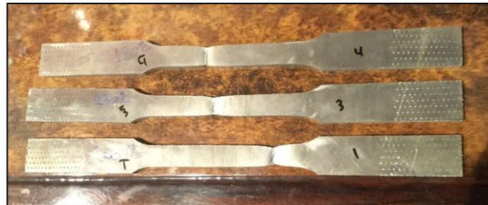
Figure 9: Specimens were tested at different temperatures.
